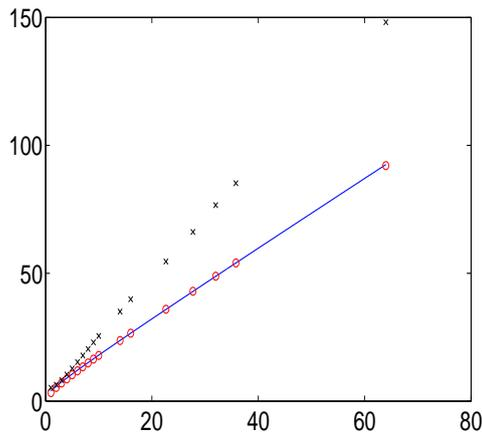
Fig 4. Drag on the segment as a function of  $Re^{1/2}$ , computed in a disk of radius 5. The blue curve is the theoretical prediction based on (8). The black crosses are the values of the drag computed with constant boundary conditions. The red circles are the values of the drag computed with second order adaptive boundary conditions.
