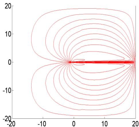
Fig 4. Non-physical back-flow induced by constant boundary conditions.
