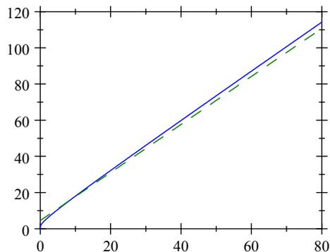
Fig. 2. Theoretical prediction of  $\frac{1}{2}C_{\text{Drag}} \text{Re}$  as a function of  $\text{Re}^{1/2}$ . The dashed green curve is the theory given by (7) and the blue curve the prediction of the triple deck theory (8).
