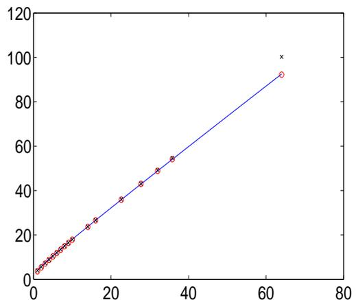
Fig 3. Drag on the segment as a function of  $\text{Re}^{1/2}$ , computed in a square of size 40. The blue curve is the theoretical prediction based on (8). The black crosses are the values of the drag computed with constant boundary conditions. The red circles are the values of the drag computed with second order adaptive boundary conditions.
